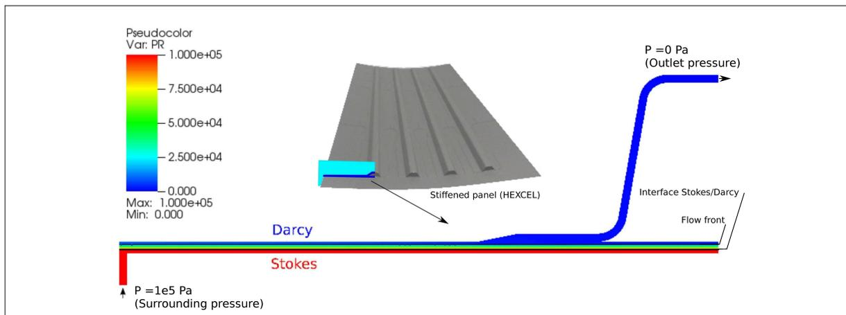
**Figure 1:** Pressure fields in macroscopic scale simulation of resin infusion manufacturing process for a slice of stiffened panel.
