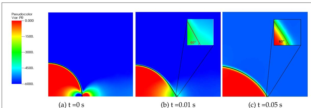
**Figure 2:** Discontinuous pressure fields in the simulation of bubble interface evolution with a contact angle of  $60^\circ$ .
